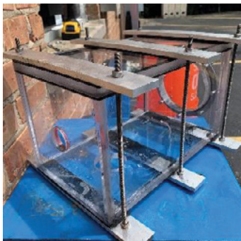
FIG A. Simple polycarbonate spray chamber—no test plate applied
