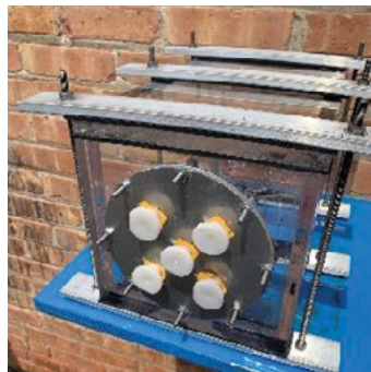
FIG B. Spray chamber rotated 180° from orientation in FIG A. Test plate installed with fastener head inside chamber. Fasteners driven into plastic bosses to represent application.
