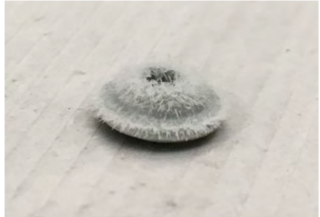
Fastener/test plate assembly at -60C
