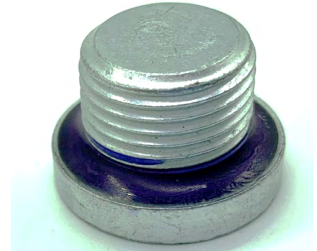
M18 Fastener Used for All Testing Zn Trivalent Finish
