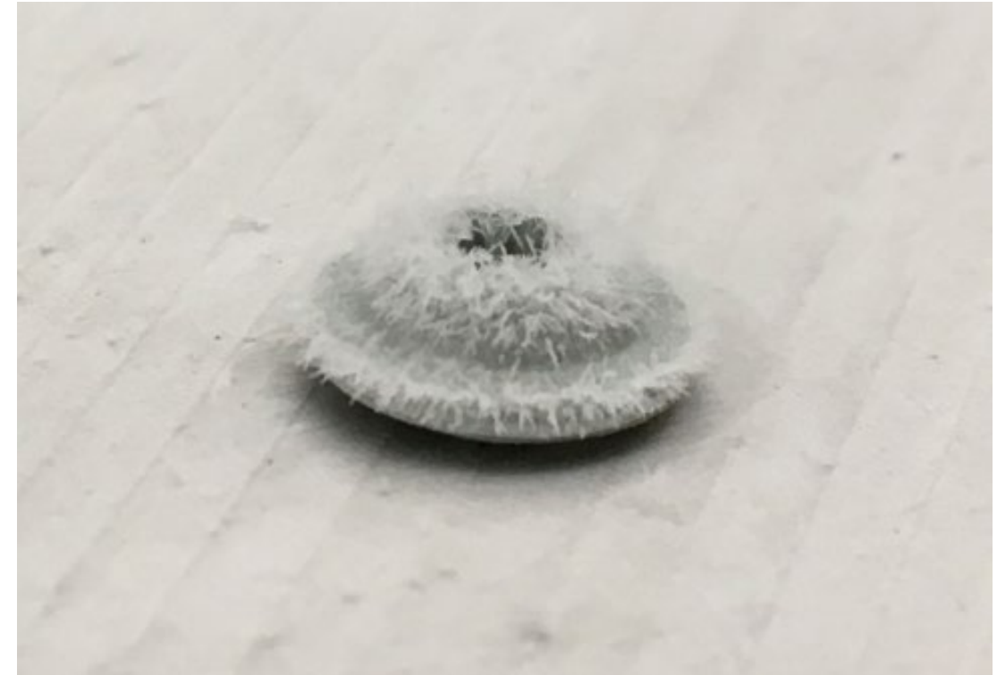
Fastener/test plate assembly at -60C
