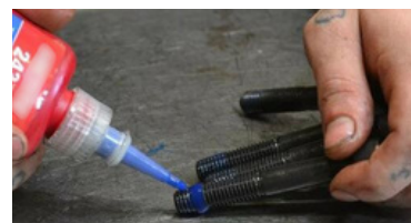
Post-Applied Application of Fastening Solution
